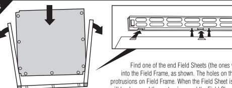
Find one of the end Field Sheets (the ones with 9 holes), and insert it into the Field Frame, as shown. The holes on the Field Sheet should match protrusions on Field Frame. When the Field Sheet is properly inserted, the holes will hook around the protrusions and the Field Sheet will not come out. Pay attention to direction, and make sure you are installing the Field Sheet right side up!
